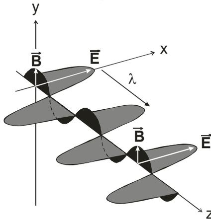
Figure 2. Schematic representation of an electromagnetic wave propagating in the direction of the z-axis. The oscillating vectors  $\vec{E}$  and  $\vec{B}$  represent the electric and magnetic fields respectively. They are always perpendicular to one another. Most of the effects of the electromagnetic wave are caused by the electric vector  $\vec{E}$ .
