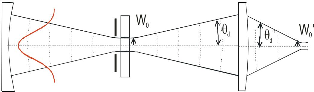
Fig. 5 The left part shows a laser cavity with an intra-cavity diaphragm for the generation of a Gaussian beam. The right part shows the propagation of the Gaussian beam through the optics. The Gaussian represents the beam intensity distribution. The dotted line represents the slightly curved wave front, e.g., the region where the electric field represented in Fig. 2 reaches its maximum. The continuous lines give the limits containing 86% of the beam power.
