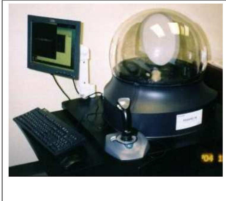
Figure 2: Perspecta 3D Volumetric Display system at The University of Tennessee at Chattanooga
