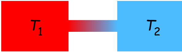
Figure 4.2 Heat exchange between two blocks of matter at different temperatures. Globally, the system receives no heat.
