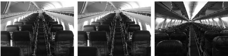
Figure 4: Embrarer 2-1 configuration (left), Embrarer 2-2 seating configuration (middle), Boeing B737 economy cabin 3-3 seating configuration.
