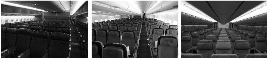
Figure 5: Boeing B777 economy class in 2-5-2 configuration (left) (photo permitted by Chris Sloan/ AirwaysNews.com ), Boeing B777 3-3-3 configuration (middle) (photo permitted by Bildarchiv der Lufthansa AG), Airbus A380 economy cabin 3-4-3 configuration (right) (photo permitted by Bernie Leighton).
